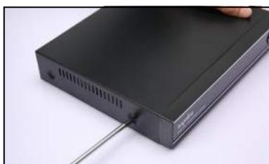
① disassemble the screw
