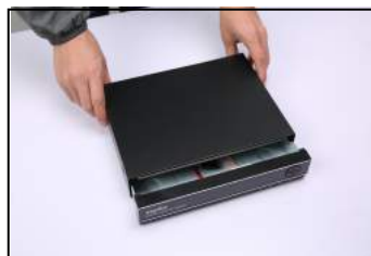
② disassemble the cover
