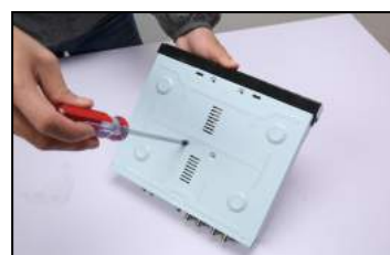
③ fix the screw of hard disk
