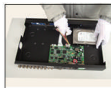
⑥ connect the power wire
