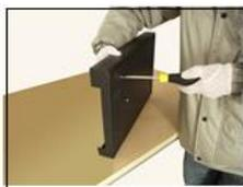
④ fix the screw of hard disk
