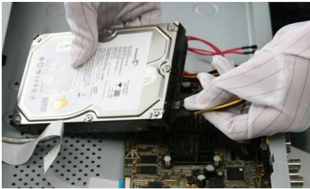
Step 4: Place the HDD on the bottom of the device and then fasten the screws on the bottom to fix the HDD.
