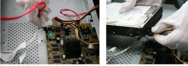
Step 3: Connect the power cable to the HDD.
