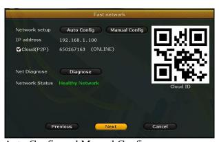
[Network Setup]: Two ways, Auto Config and Manual Config.
