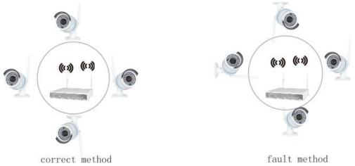
The signal coverage of Antenna is similar to a round circle. Antenna located in center of the round circle, signal of surrounding is much stronger, but much weaker if antenna endpoints backoff direction. And in order to guarantee the video quality, IPC antenna should try to keep in parallel or tangent with NVR
