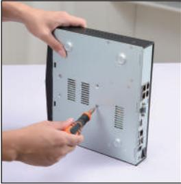
④ fix the screw of the hard disk
