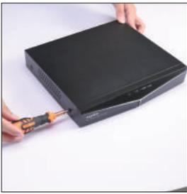
① disassemble the screw
