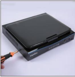
① disassemble the screw
