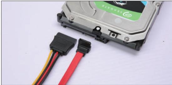
► Connect the data wire and the power wire to the corresponding port of the hard disk
