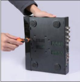
④ fix the screw of hard disk
